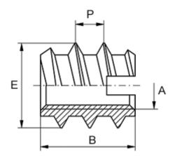
Female thread A = M3Length B = 6Male thread E = 6.0Min hole depth = 8Recommended bore diameter (plastic/hard wood) = 4.2 to 4.3Recommended bore diameter, soft wood (largest) = 4.0Thread pitch P = 2.0
